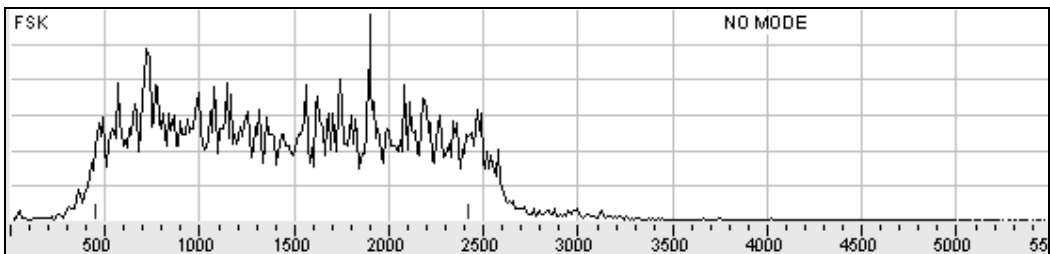
Picture 420: Spectrum of digital NBTV
