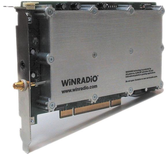
The WinRADIo WR-G313i receiver is a software-defined high-performance HF receiver (9 kHz to 30 MHz, optionally extendable to 180 MHz) on a PCI card. The front-end is a DDS-based double-conversion superhet, the last IF stage is implemented in software resident in the on-board DSP.
