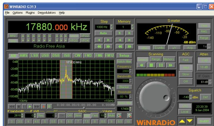
The receiver is extremely sensitive, making it possible to comfortably read CW signals well under -130 dBm input levels, yet featuring a respectable 95 dB dynamic range making the receiver resistant to strong signal overload.
