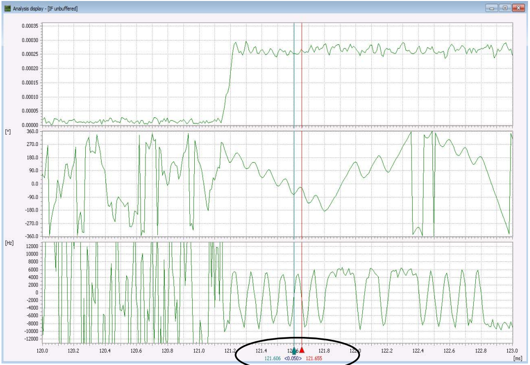
Picture 136: Baud rate measurement of one hop
