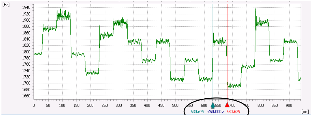
Picture 73: Tone duration measurement with MFSK oscilloscope
