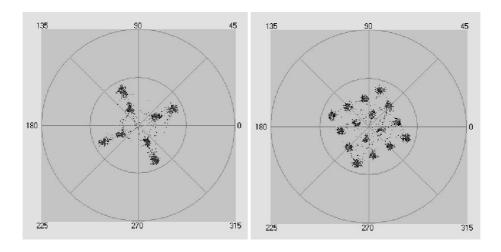
Picture 14: example of an 8QAM and 16QAM in the Phase Plane
