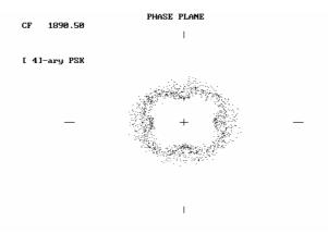
Picture 12: Phase plane of a OQPSK
